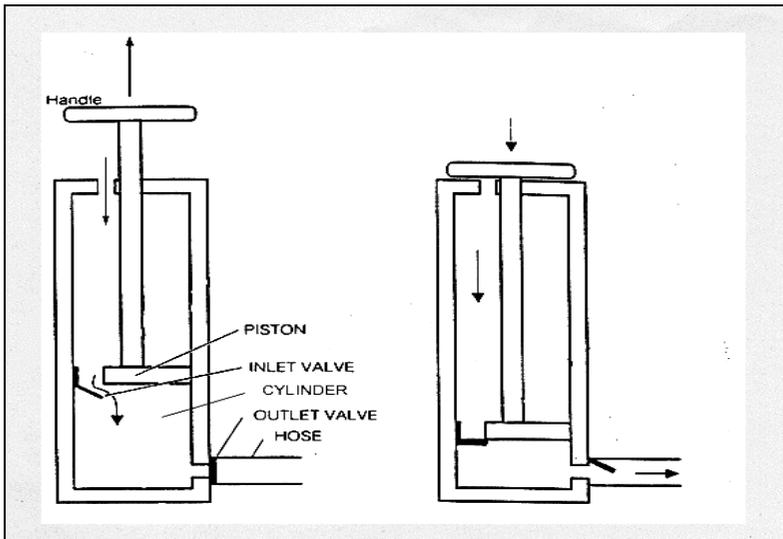
Fig. 3: Diagram of bicycle pump with arrows
