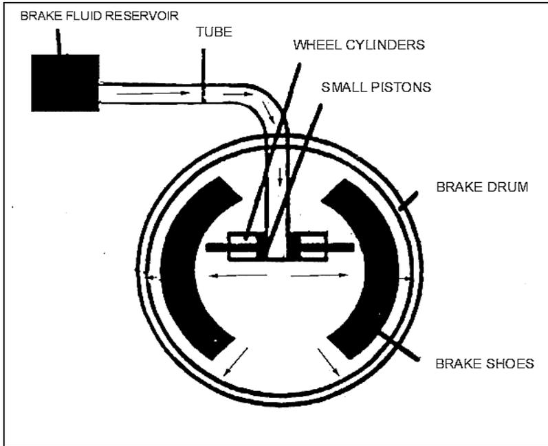
Fig. 4: Diagram of a car brake with arrows
